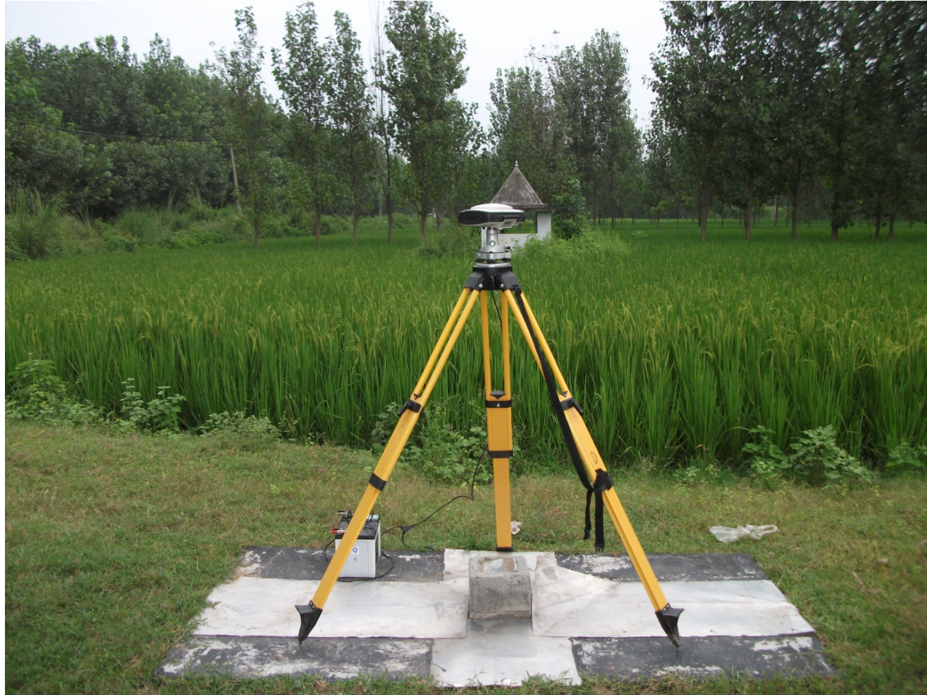
DGPS machine installed on primary point
