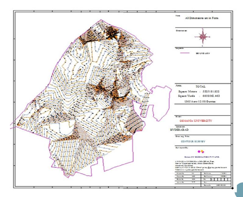
Figure 5. One meter contour map of the watershed along with the spot heights
