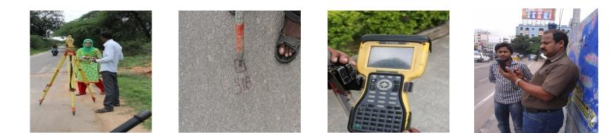
Figure.4\_Identifying the spot heights to create a contour map using the Total Station and DGPS.
